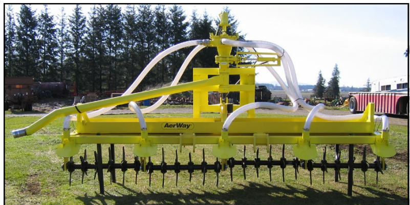
Rear view shows swinging tube, and splash plates
